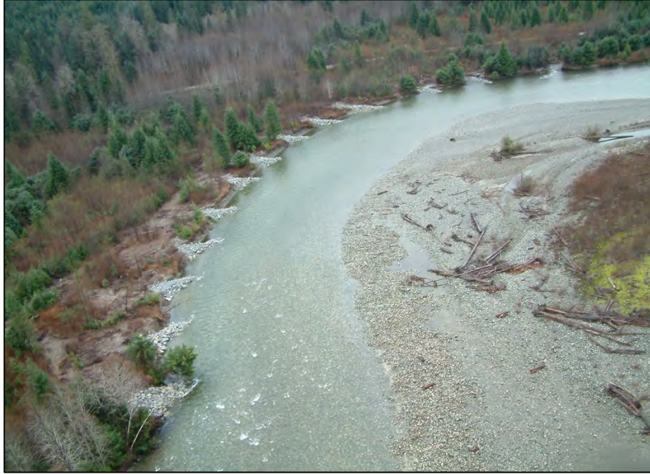
Photo 6. Rock groynes constructed on an eroding left bank in the Phillips River.
